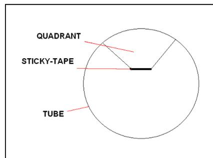
Figure 4.1 Cross-section diagram of tube design (front entrance).
